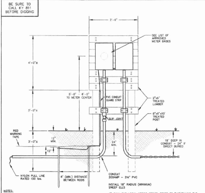
1) RUN THE CONDUIT FROM THE POLE, PEDESTAL, OR PADMOUNTED TRANSFORMER; WRECC WILL INDICATE THE BEGINNING POINT FOR THE CONDUIT WITH A WOODEN STAKE MARKED "CONDUIT TO HERE". IF STAKE IS ON POWER POLE, EXTEND CONDUIT 1'-0" ABOVE GROUND AND STRAP TO POLE. CAP OR CLOSE OPEN ENDS OF CONDUIT. INSTALL RED WARNING TAPE 12 INCHES ABOVE CONDUIT.
